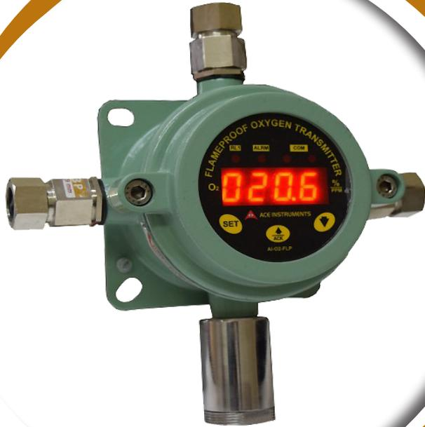
Flameproof Oxygen Monitor Transmitters manufactured by Ace Instruments are high precision microcontroller based gas transmitters housed in flameproof aluminum LM-6 Body certified by CIMFR, Dhanbad for use in Gas Group Areas I, II, IIA & IIB. The 4 digit LED display shows the digital display of oxygen gas concentration in the range of 0.0 to 25.0% Volume.
